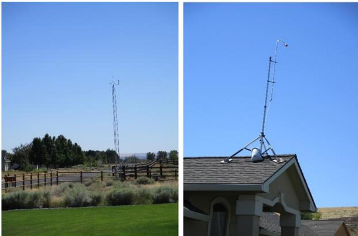
**Figure 4.4.** Left photograph shows the 10-m meteorological tower at the Horn Rapids site. Photo shows view looking south. Right photo shows air sampling inlet mounted on a tripod on the property owner's roof. Teflon tubing conveyed air to instruments located in a room inside the house.
