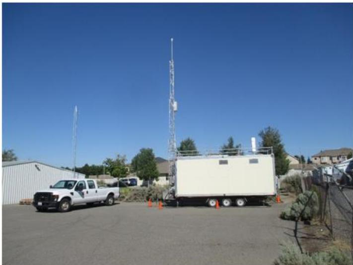
**Figure 4.2.** Photograph of the MACL equipment shelter at the BCAA location on July 28, 2016 for the T-COPS study. The MACL is equipped with a telescoping mast that provided a support tower for a surface meteorological weather station visible at the top of the mast as well as inlets for air sampling.
