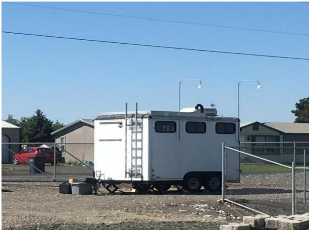
**Figure 4.5.** Burbank trailer with instruments and inlets installed. Inlets were located approximately 4-m above ground level and 1-m above the trailer roof.
