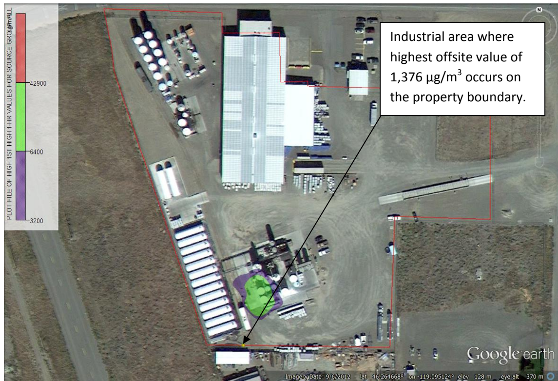
Diagram 21: 1 st High – 2 Hour Concentrations of Ammonia (Comparison to ATSDR Value of 1,184 \mu\text{g}/\text{m}^3 )
