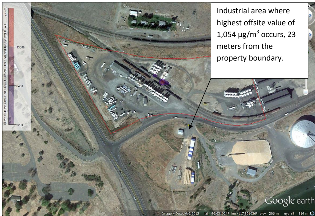
Diagram 8: 1 st High – 2 Hour Concentrations of Ammonia (Comparison to ATSDR Value of 1,184 \mu\text{g}/\text{m}^3 )
