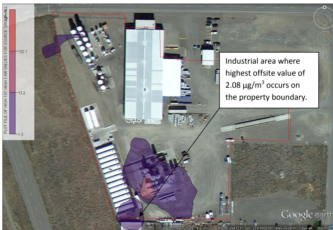
Diagram 19: 1 st High – 1 Hour Concentrations of Fluoride (Comparison to NRC Value of 1,321 \mu\text{g}/\text{m}^3 )
