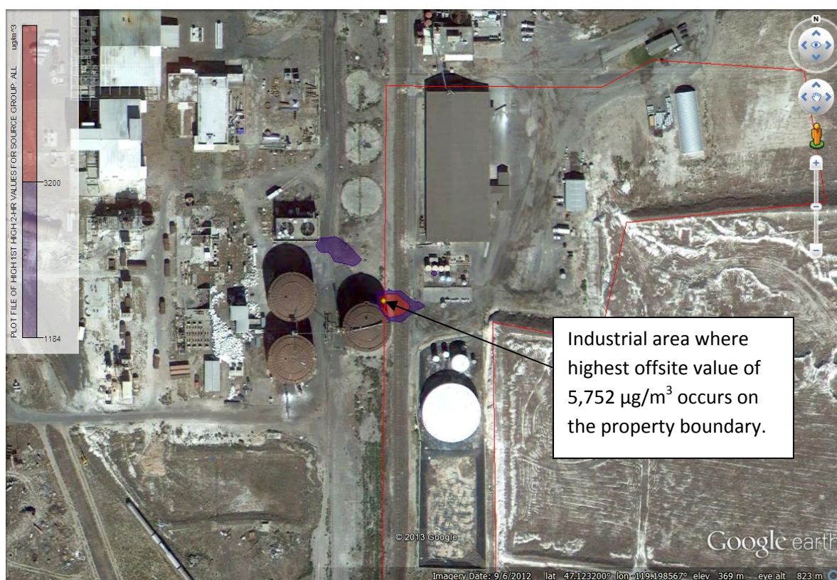
Diagram 15: 1 st High – 2 Hour Concentrations of Ammonia (Comparison to ATSDR Value of 1,184 \mu\text{g}/\text{m}^3 )
