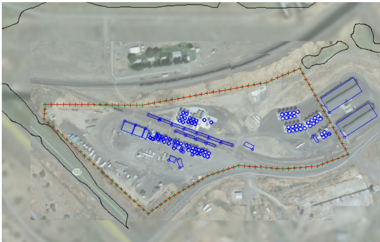
Diagram 3: Structures Considered for Downwash
