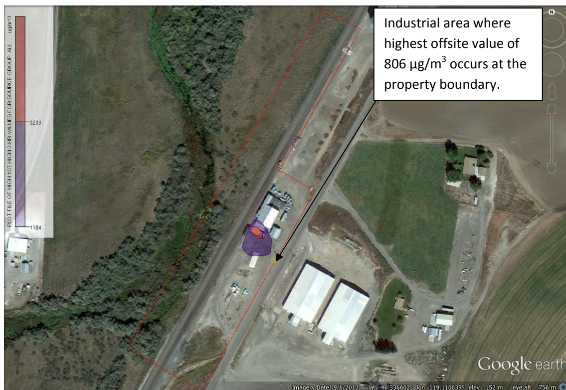
Diagram 18: 1 st High – 2 Hour Concentrations of Ammonia (Comparison to ATSDR Value of 1,184 \mu\text{g}/\text{m}^3 )
