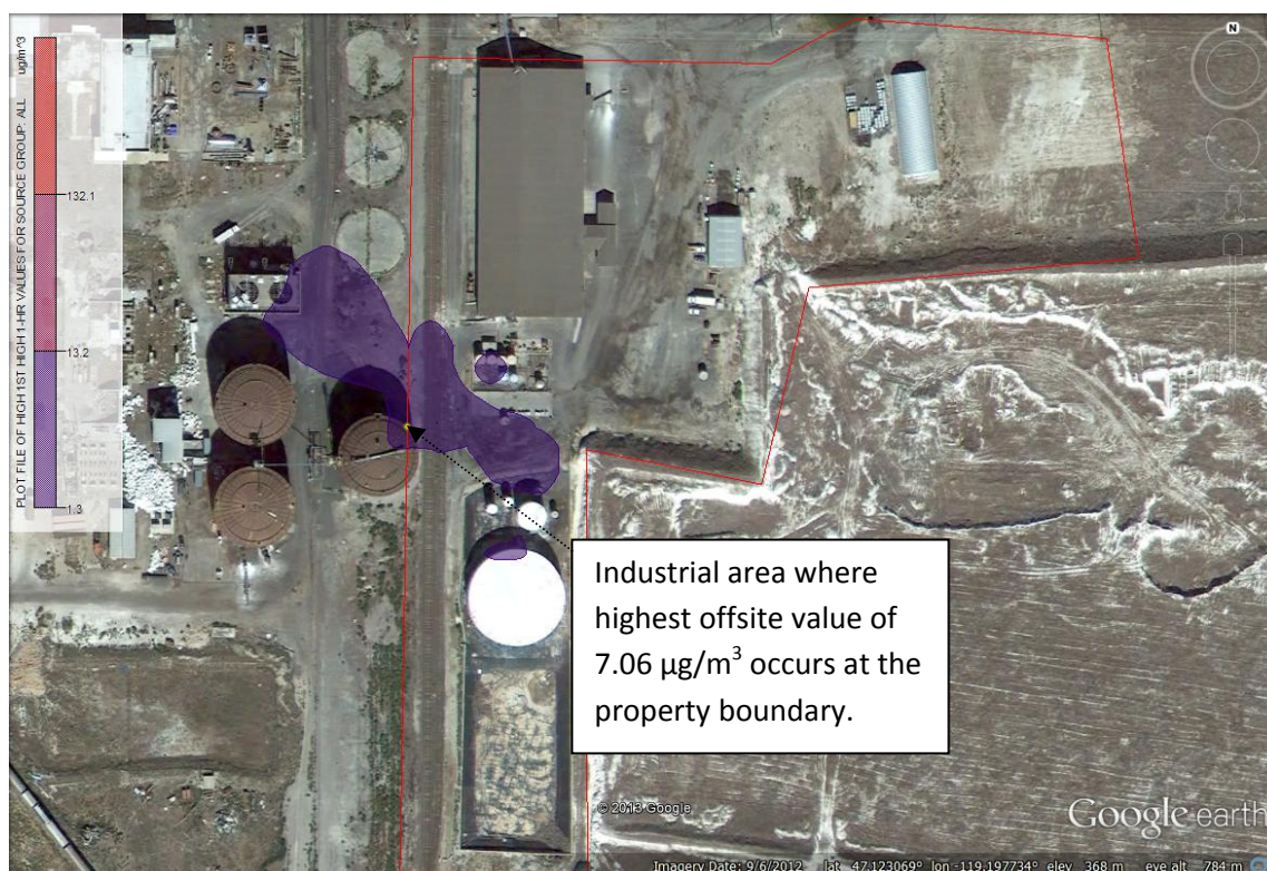
Diagram 12: 1 st High – 1 Hour Concentrations of Fluoride (Comparison to NRC Value of 1,321 \mu\text{g}/\text{m}^3 )
