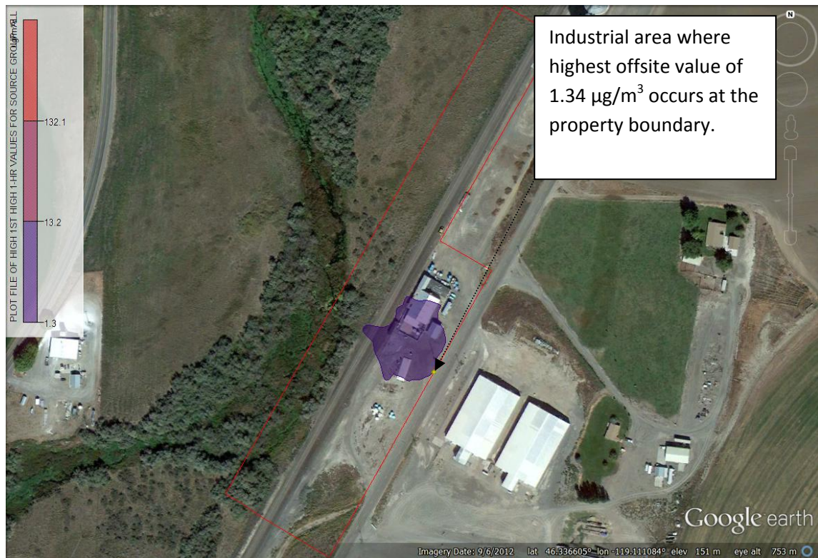
Diagram 17: 1 st High – 1 Hour Concentrations of Ammonia (Comparison to Cal OEHA Value of 3,200 \mu\text{g}/\text{m}^3 )
