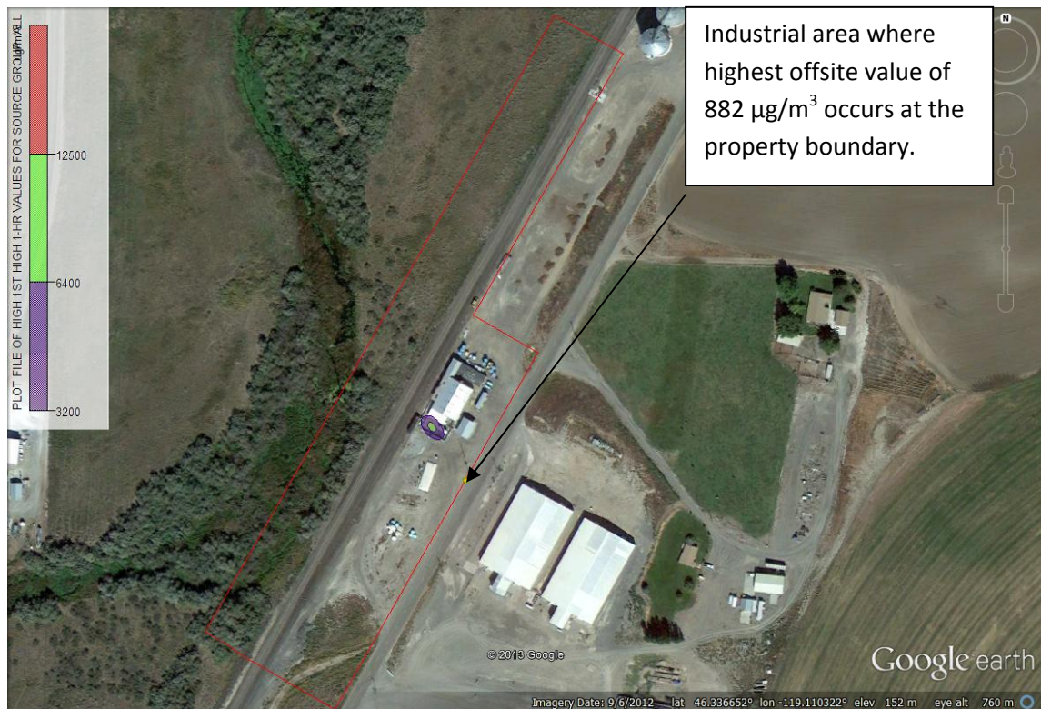
Diagram 17: 1 st High – 1 Hour Concentrations of Ammonia (Comparison to Cal OEHA Value of 3,200 \mu\text{g}/\text{m}^3 )
