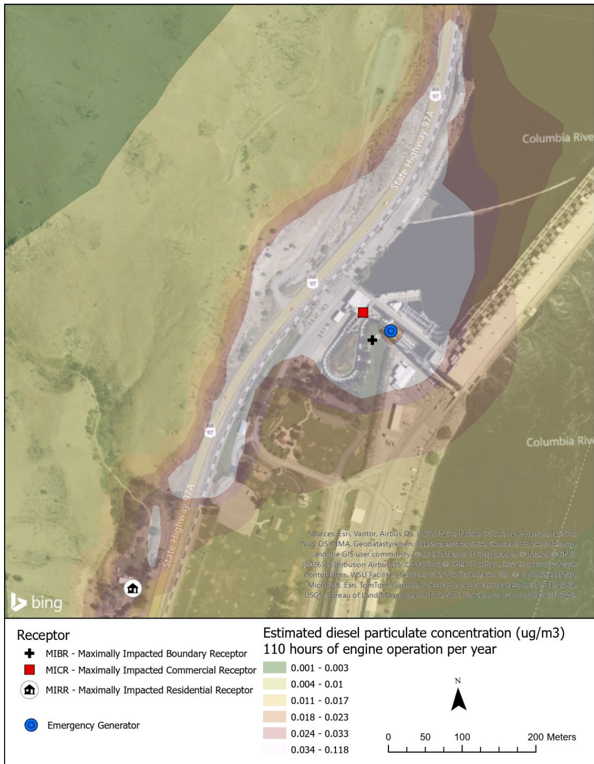
Figure 1: Estimated average diesel particulate concentration from emergency generator operation
