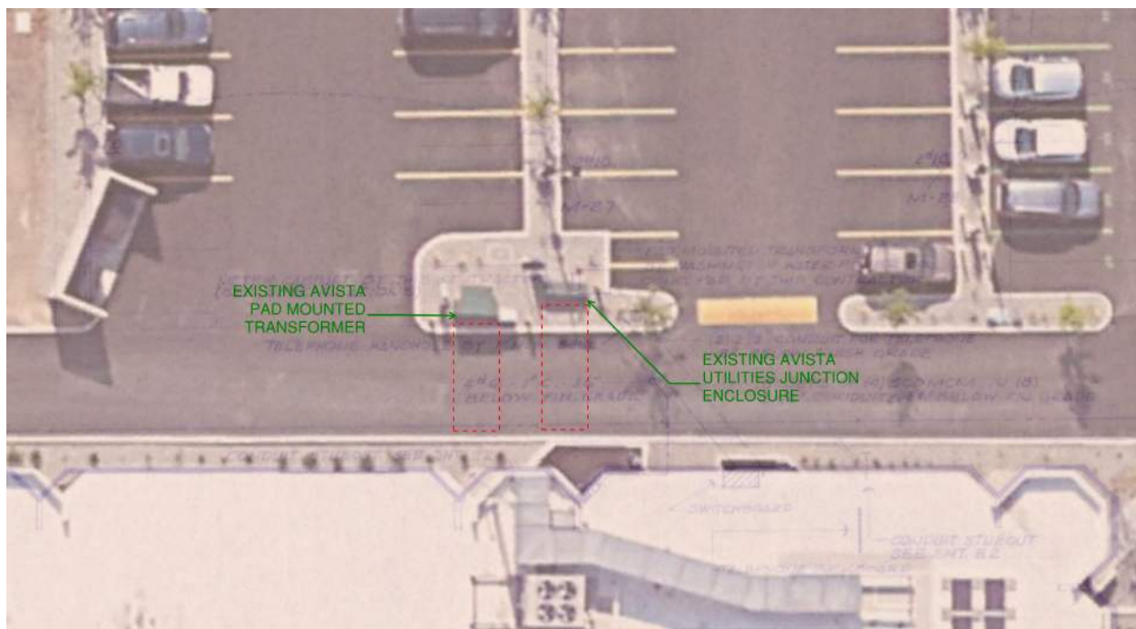
Figure 1 – Existing Avista Utilities Pad-Mounted Transformer and Junction Enclosure
