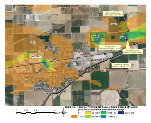
**Figure 11.** Number of hours/year that NO<sub>2</sub> levels could exceed 441  $\mu$ g/m<sup>3</sup> (assuming continuous outage conditions)
