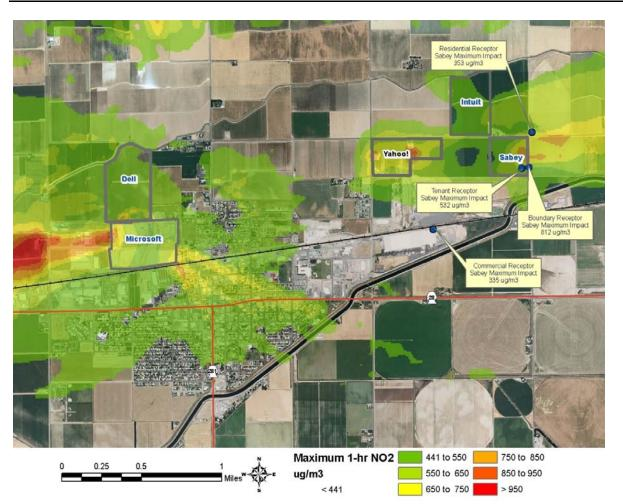
Figure 10. Maximum cumulative 1-hour NO<sub>2</sub> levels assuming simultaneous outage emissions
