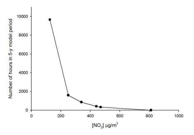
**Figure 14.** Number of hours per year the 1-hour average NO<sub>2</sub> concentration would have reached 441  $\mu$ g/m<sup>3</sup> given concentrations at the MIBR if the Sabey Quincy Data Center generators had run continuously from the beginning of 2004 to the end of 2008
