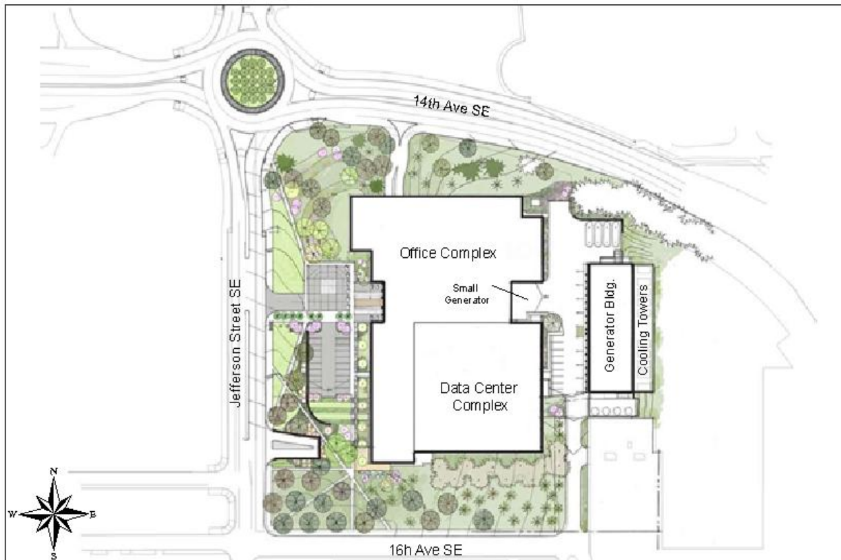
Figure 2. Proposed DIS site plan showing general location of air emission units (adapted from Wright Runstad, 2009)
