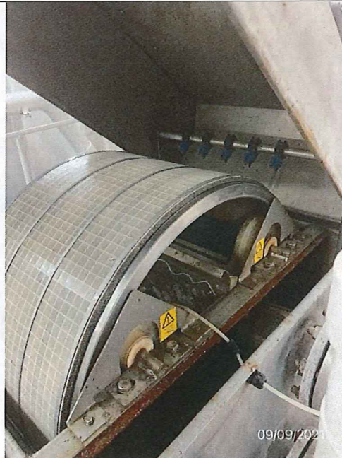
Photo # 16 Image: IMG_0233 Date: 9/9/2021 Taken by: Evan Dobrowski Description: Scanship polishing filters - inside
