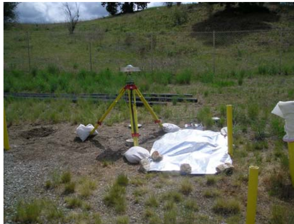
Figure 5. GPS base station at the abandoned Liberty Lake landfill.
