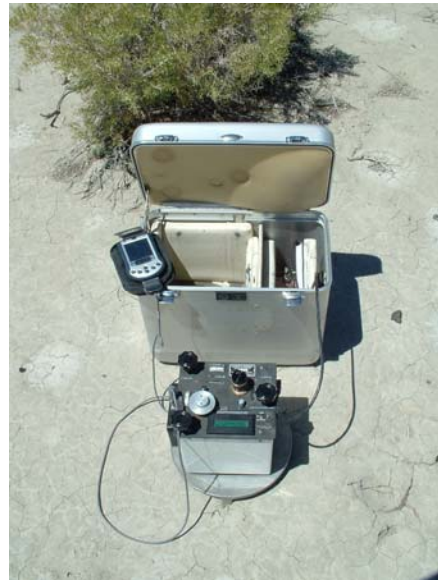
Figure 7. LaCoste-Romberg G meter with Aloid upgrade (meter G1069) used in gravity acquisition.
