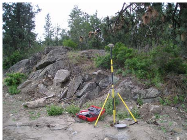
Figure 6. GPS rover used to located gravity stations.
