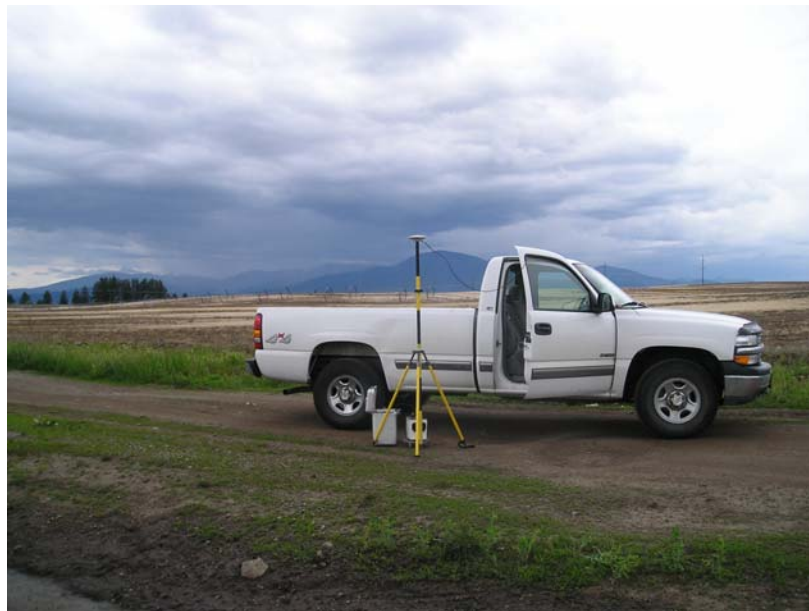
Figure 8. Typical measurement configuration showing gravimeter and GPS positioning.
