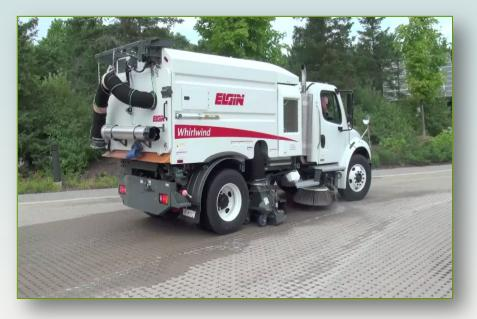
Vacuum settings may have to be adjusted to prevent excess uptake of aggregate from paver openings or joints. Vacuum surface openings in dry weather to remove dry, encrusted sediment.
