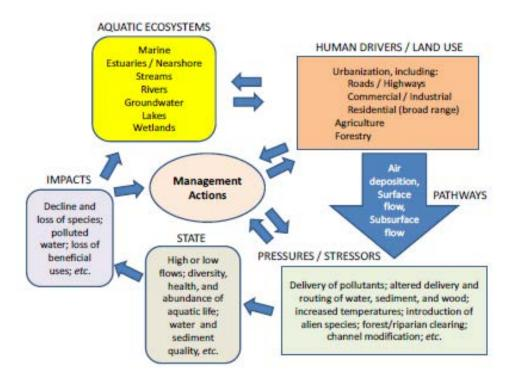
Figure 1: Stormwater Stressors and Pathways
