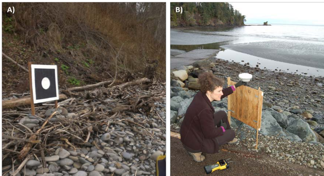
Figure 6. A) Photo showing a plywood target setup for ground control during the boat-based LiDAR survey. B) Photo showing the use of a Trimble R8 GNSS receiver to obtain the position of a ground control target.
