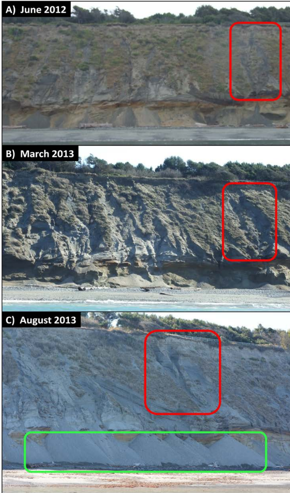
Figure 18. Digital photos taken during each of the three boat-based LiDAR surveys; used to qualitatively verify the results of the difference surfaces shown in Figure 19.
