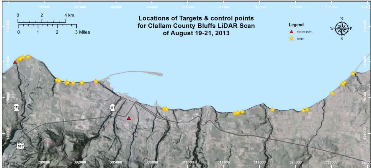
Figure 5. Map of study area showing locations of targets setup for ground control during the third boat-based LiDAR survey in August 2013, as well as benchmarks surveyed as control points.
