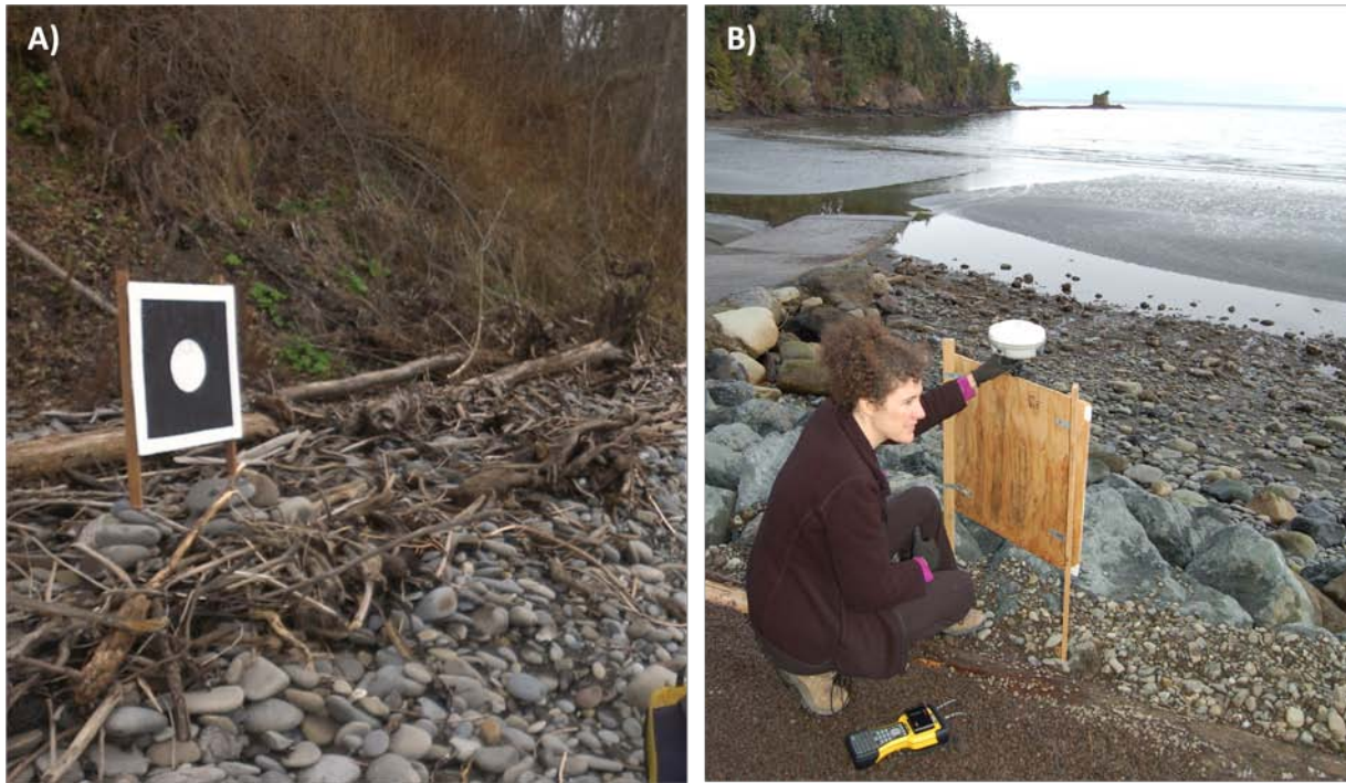
Figure X. Photos showing plywood targets installed and surveyed in as a ground control points for the laser point cloud.
