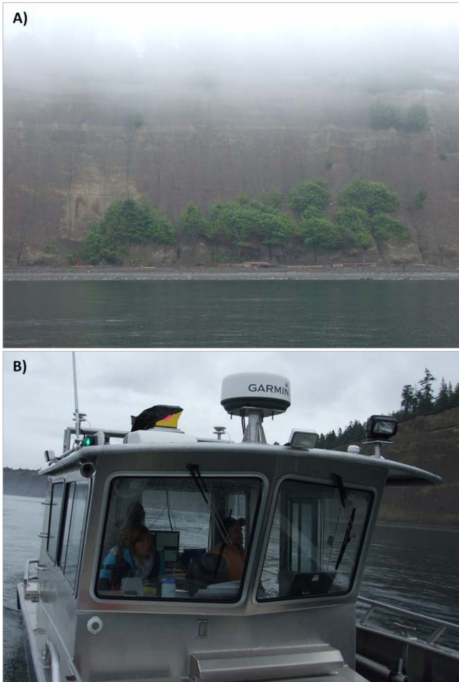
Figure X. Adverse weather conditions complicating the survey. A) Foggy conditions obscuring bluff top. B) As a precaution, the laser scanner was partially covered with a garbage bag due to light rain.
