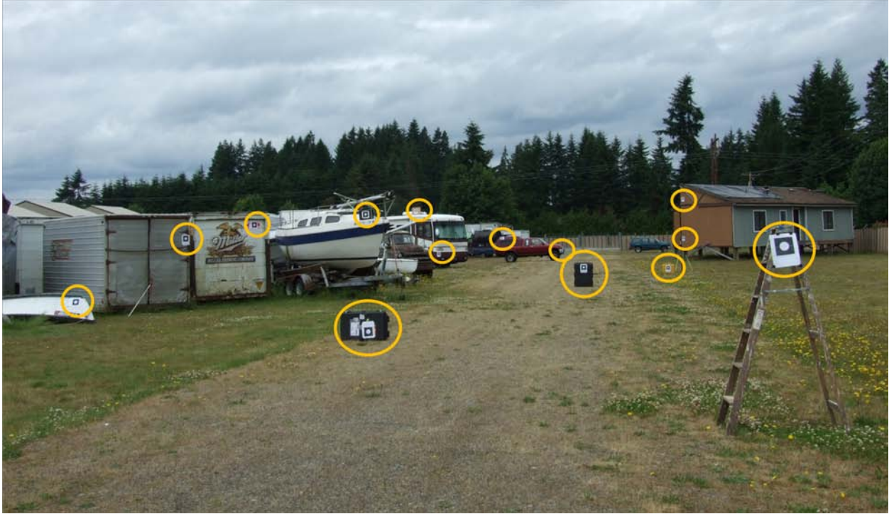
Figure 3. Placement of 14 targets within the laser scanner's field of view, at varying heights and distances.
