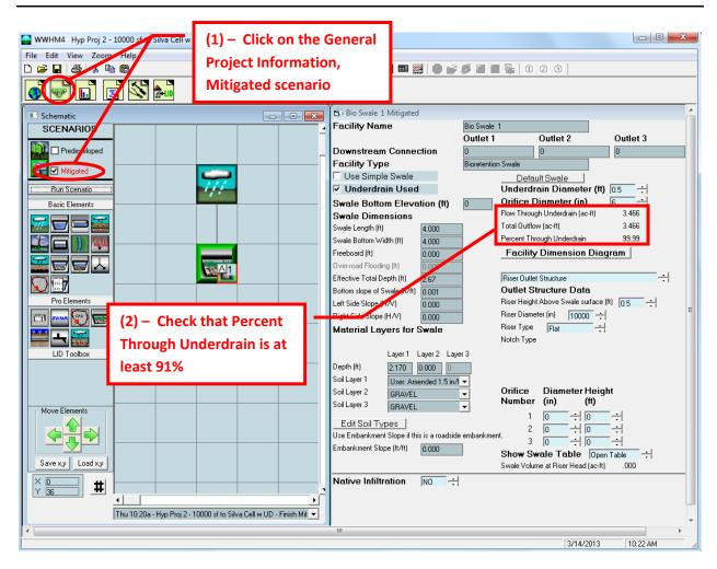
The resulting length that passed the treatment requirement was 4 feet in this example. Note that this is approximately one-tenth the length that is available for Silva Cells based on the Project Example assumptions.
