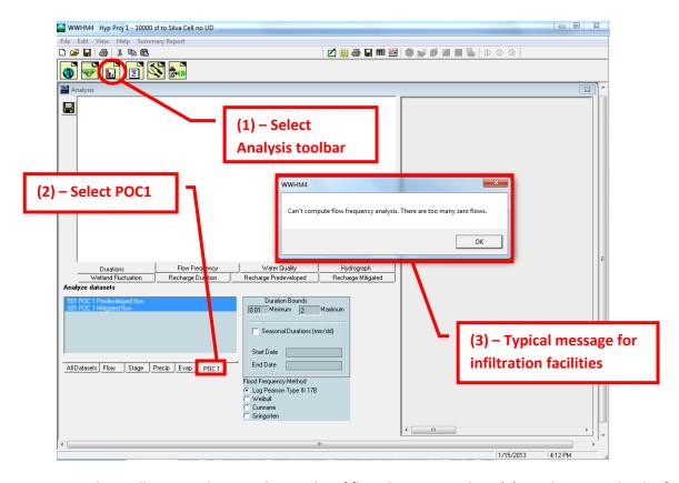
A window will pop up showing the results of flow duration analysis (4). In this example, the facility passes as-is. If the facility does not pass, change the design and re-run the model until a passing result is obtained.
