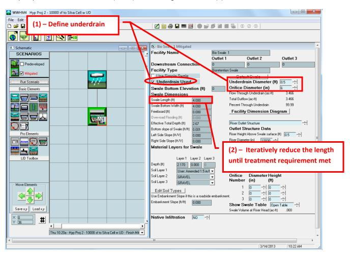
Navigate back to the General Project Information tab and select the Mitigated schematic (1). Re-run the Mitigated scenario with the new Silva Cell configuration. Left click the bioretention element. Model results will populate the space beneath the underdrain input (2). Check that the Percent Through Underdrain is at least 91%.
