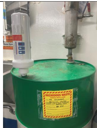
Photo #08 5/8/23 Image: IMG_183 By: Dobrowski Description: Aerosol Can Filtration
