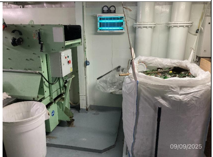
Photo # 10 Image: IMG_3120 Date: 9/9/2025 Taken by: Evan Dobrowski Description: Photo of food pulper/biodigester
