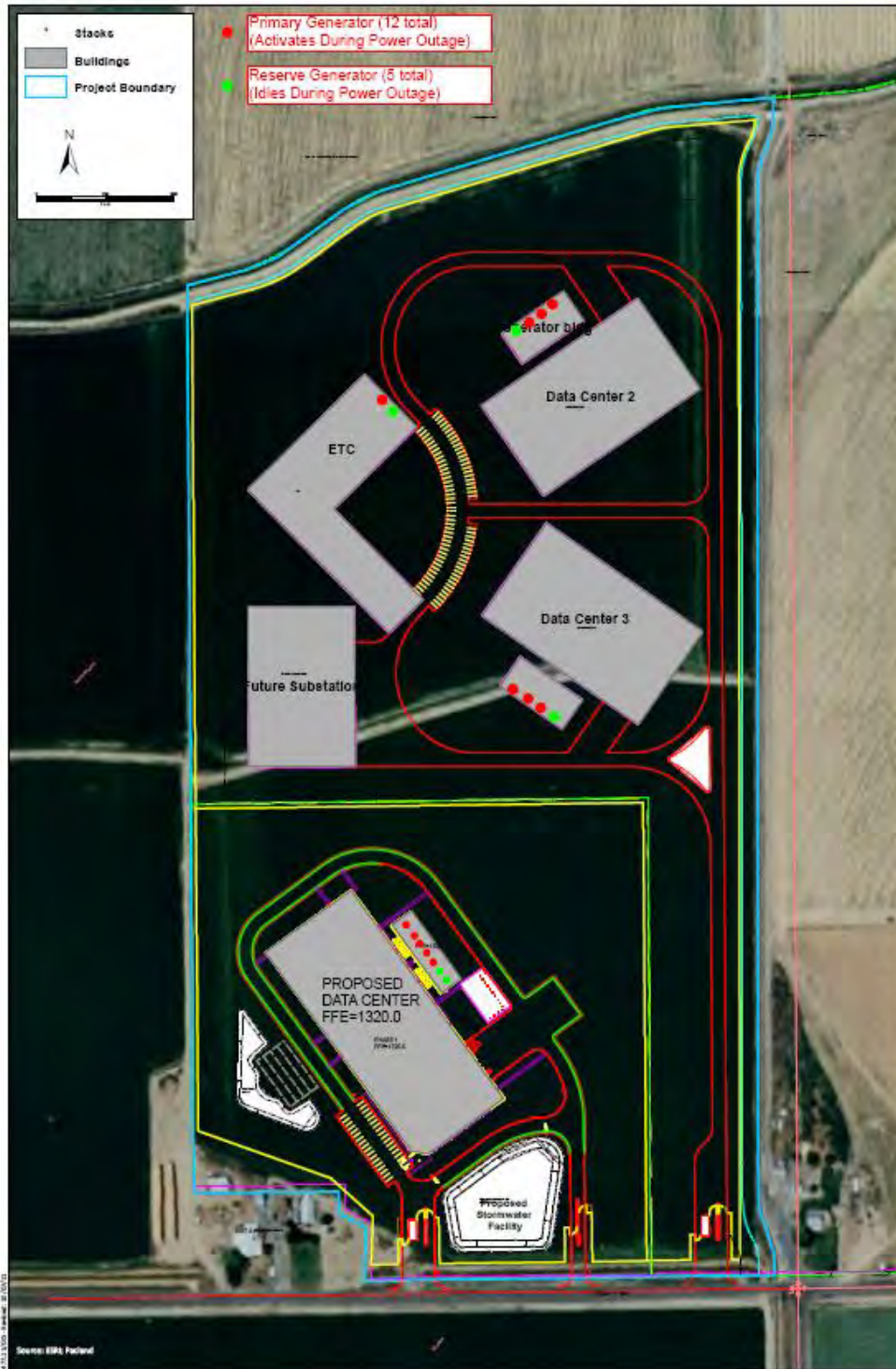
Figure 2-2. Site Layout for the Vantage Data Center
