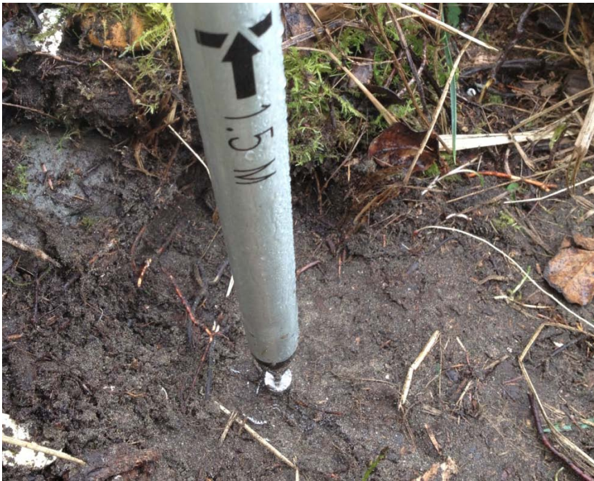
Figure 12. A finished rod monument sits almost flush with the ground and has a small divot drilled in the center to hold a tripod tip. Each rod marker has feet of aluminum or steel rod beneath the surface.
