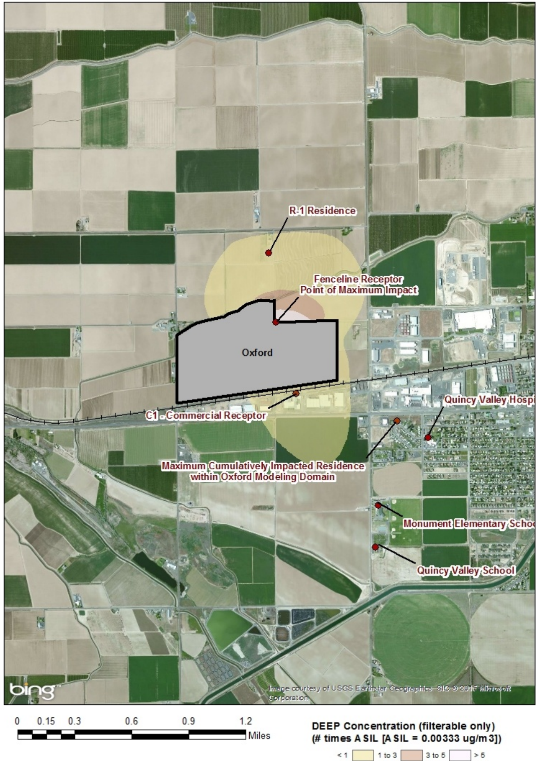
Figure 3. Receptor locations in relation to estimated DEEP concentrations (assuming only filterable fraction represents DEEP). Concentrations are reported as the number of times higher than the ASIL.
