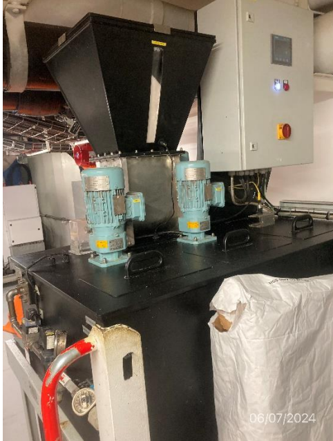
Photo # 37 Image: IMG_1708 Date: 6/7/2024 Taken by: Evan Dobrowski Description: Flocculant hopper and mixing tank
