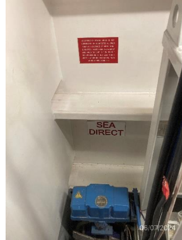
Photo # 34 Image: IMG_1705 Date: 6/7/2024 Taken by: Evan Dobrowski Description: Sewage overboard valve in the closed position
