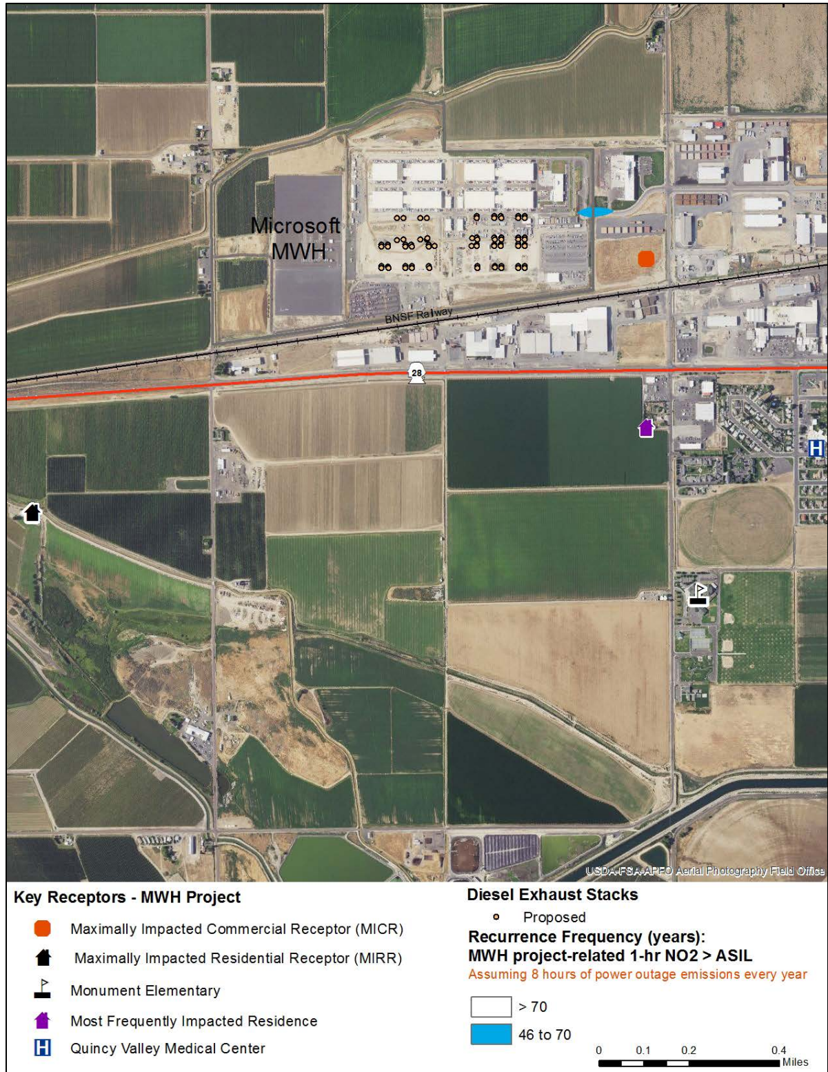
Figure 7: Estimated time interval (years) between occurrences of 1-hr NO 2 concentrations greater than 454 µg/m 3 assuming eight hours of MWH-03/04/05/06 data center emergency engine outage emissions per year
