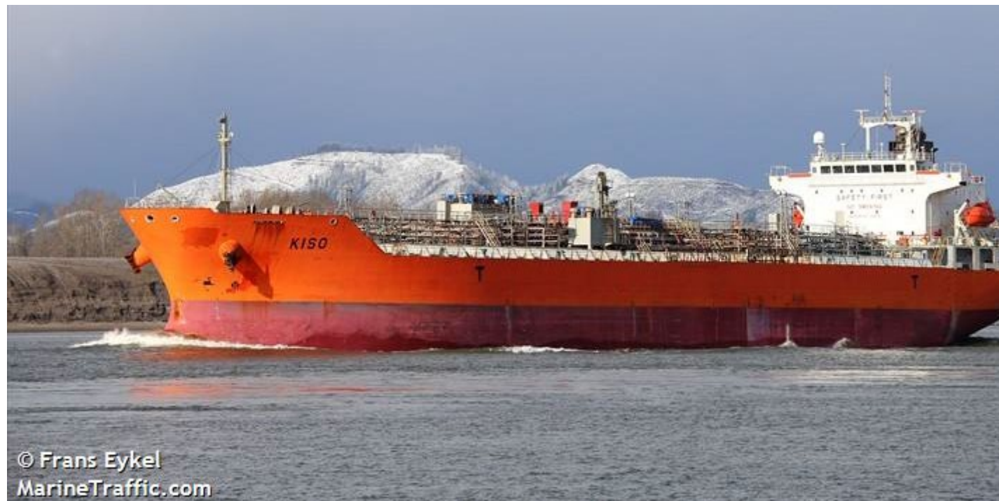
An oil/chemical tanker. This example is 557 feet long, 33,600 DWT, and can carry 10 million gallons of oil.
