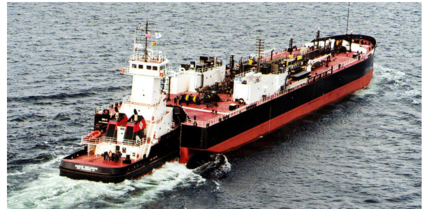
An articulated tug and barge (ATB). This example is 480 feet long, 18,000 DWT, and can carry 6.7 million gallons of oil.
